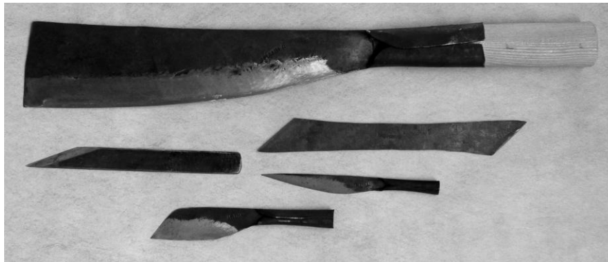
Figure 56 Vietnamese bamboo knives. The large knife is the principal kite bamboo knife
